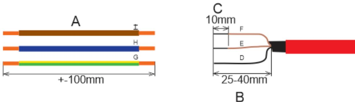
1. Strip back (A) the outer insulation of the cold tail & cut off about 100mm of (non-resistive wire) brown(I), blue(H) & earth(G) wire. On each of these lengths, strip off the insulation to expose about 10mm of copper at each end
